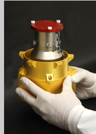
RAD "Radiations Assessment Detector", 1.5Kg © NASA
